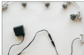
5. Insert power line set (LL1 socket+Power Line)
